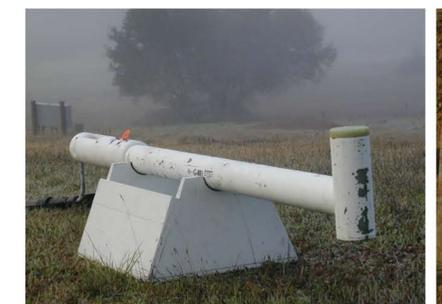
Figure 6: total-field magnetometer at JRSC
