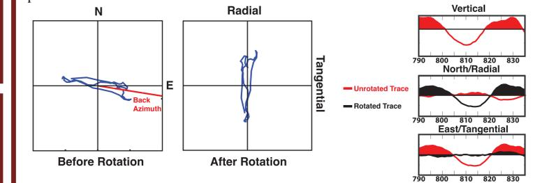
**Figure 5:** Particle motion of a representative trace from the 3C dataset. Green line on diagram represents back azimuth of station from shot 31. Seismograms showing original traces (red) and rotated traces (black).
