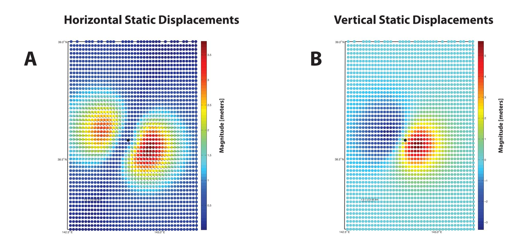
Fig. A: Horizontal residual displacements of the seafloor above the source (colors are absolute magnitude). Fig. B: Vertical residual displacements of the seafloor above the source.
