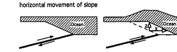
in which H is the water depth and  $u_X$  and  $u_Y$  are the horizontal displacements due to faulting (Tanioka & Satake, 1996).
