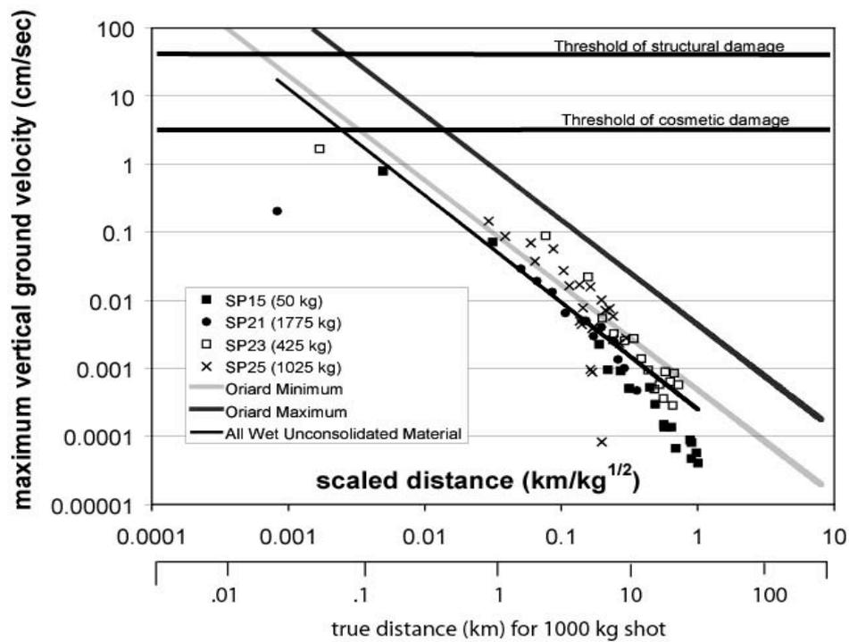
**Figure 4.** Maximum vertical ground velocities for borehole shots in wet unconsolidated material. The 'All wet unconsolidated material' trendline shows the best-fit curve of the Oriard form to our EAGLE data.
