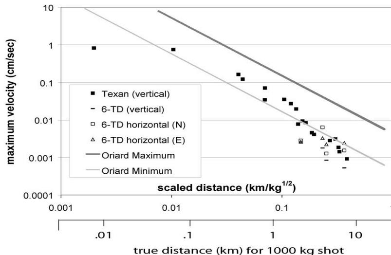
**Figure 1.** Maximum ground velocities from short-period and broadband three-component sensors for a single shot.
