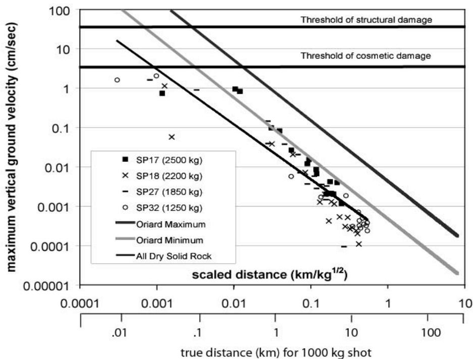
**Figure 5.** Maximum vertical ground velocities for borehole shots in dry solid rock. The 'All dry solid rock' trendline shows the best-fit curve of the Oriard form to our EAGLE data.
