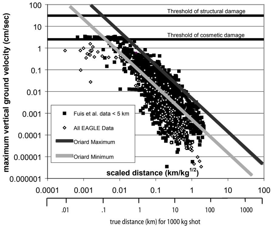
**Figure 2.** Maximum vertical ground velocity from short-offset LARSE II and EAGLE data. Threshold for cosmetic and structural damage from Nicholls et al. (1972).
