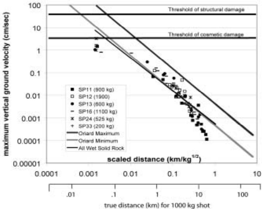
**Figure 3.** Maximum vertical ground velocities for borehole shots in wet solid rock. The 'All wet solid rock' trendline shows the best-fit curve of the Oriard form to our EAGLE data.
