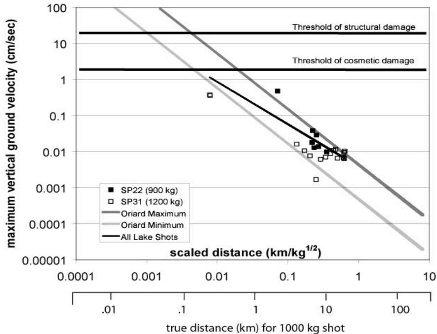
**Figure 6.** Maximum vertical ground velocities for lake shots. SP 22 was fully confined and fired at the optimum depth of 87m in Lake Shala. SP 31 was only partially confined (it produced water boils) - it was fired in a shallower lake (Arenguade) on the lake bed at 31 m. The 'All lake shots' trendline shows the best-fit curve of the Oriard form to our EAGLE data.
