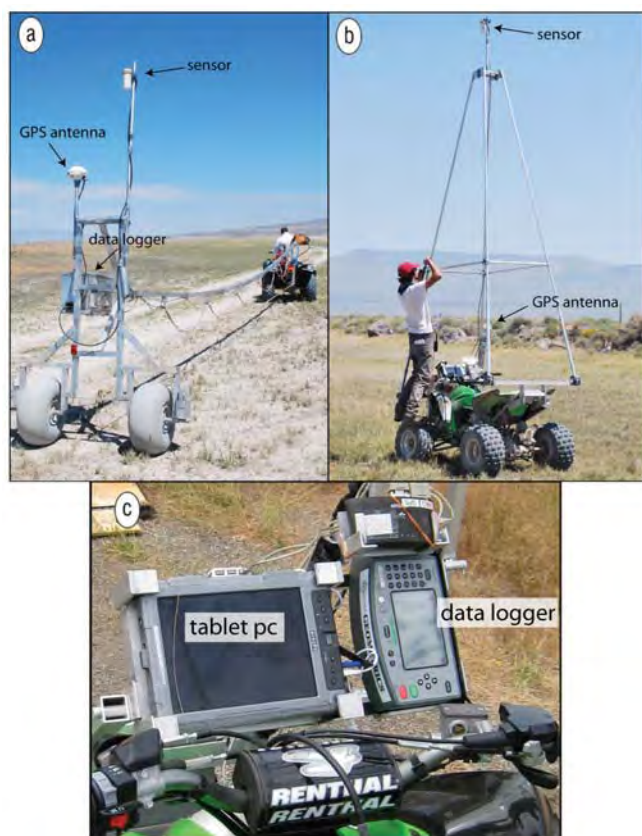
Figure 1. (a) The towed system. The magnetometer sensor and GPS antenna are on an aluminum carriage that is towed 9 m behind the ATV. (b) The tower system. The magnetometer sensor is placed 3.6 m directly above the ATV and the GPS antenna is on the front of the ATV. (c) Ruggedized tablet PC and data logger on the tower system. Magnetic readings and GPS locations are streamed in real time to the tablet PC via a Geometrics data-logger console.
